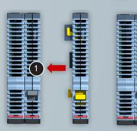
The positive "click-to-lock" mechanism firmly clamps Flexslice modules to each other to form a Flexslice station. Simply push each module together and slide the quick release locks into position.
