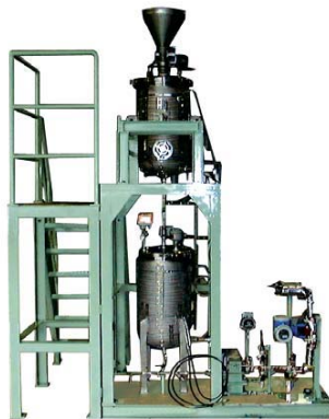
With two tanks and a flow meter.
